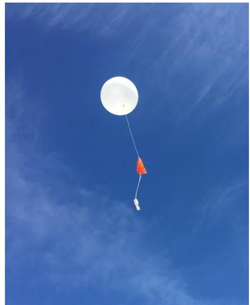
**Launching radiosondes upwards**
